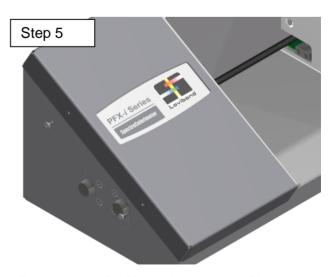
Replace the left lid by replacing the 2x M3 x 8 socket head screws.
