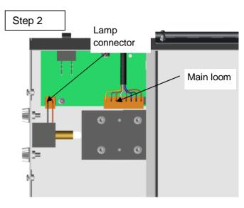
Disconnect the Lamp Holder Assembly connector and the Main Loom connector from the Power Board.
