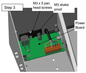
Remove the Power Board by removing the 4x M3 x 6 pan head screws and 4x M3 shake proof washers.
