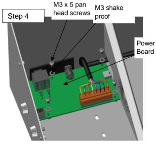
Replace the Power Board by replacing the 4x M3 x 6 pan head screws and 4x M3 shake proof washers.
