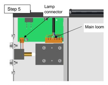
Replace the Lamp Holder Assembly connector and the Main Loom connector to the Power Board.
