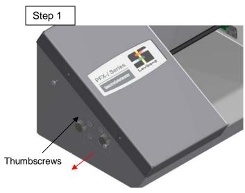
Remove the lamp holder by unscrewing the two thumbscrews on the side of the cabinet
