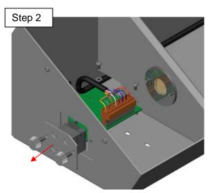
Pull the lamp holder assembly out of the cabinet..
