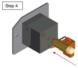
Screw in the new lamp. Do not touch the glass lens on the lamp, as fingerprints will impair its performance
