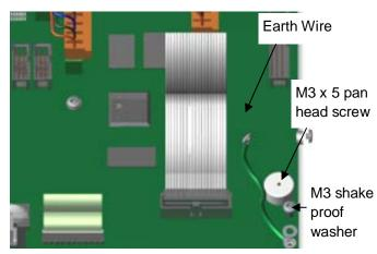
Attach the Earth Wire to the Main Board using 1x M3 x 5 pan head screw and 1x M3 shake proof washer as shown.
