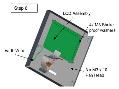
Replace the new LCD Assembly using 3x M3 x 10 pan head screws and 3x M3 shake proof washers as shown. Attached the Earth Wire (137390) in the bottom left corner using 1x M3 x 10 Pan head screw and 1x M3 shake proof washer.
