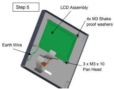
Remove the LCD Assembly from the inside of the right lid by unscrewing the M3 x 10 pan head screws and the M3 shake proof washers as shown.
