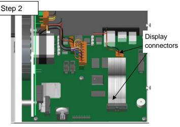
Remove the Display connectors from the connectors on the Main boards as shown.
