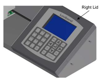
Replace the right lid carefully by replacing the 2x M3 x 8 pan head screws
