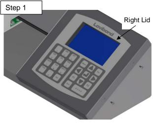
Remove the right lid carefully by removing the 2x M3 x 5 pan head screws
