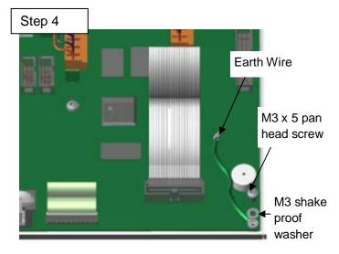
Disconnect the Earth Wire from the Main Board using 1x M3 x 5 pan head screw and 1x M3 shake proof washer as shown.
