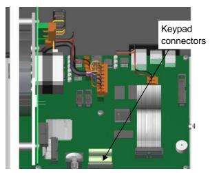
Replace the keypad connector to the connectors on the Main Boards as shown.
