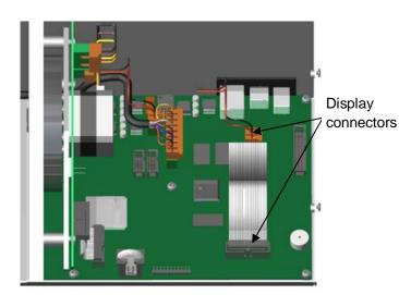
Attach the Display connectors to the connectors on the Main boards as shown.
