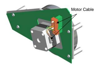
Reconnect the motor cable to the motor and the Motor Board.
