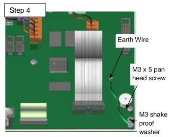
Remove the Earth Wire from the Main Board by removing the M3 x 5 pan head screw and the M3 shake proof washer as shown.
