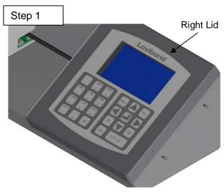
Remove the right lid carefully by removing the 2x M3 x 5 pan head screws
