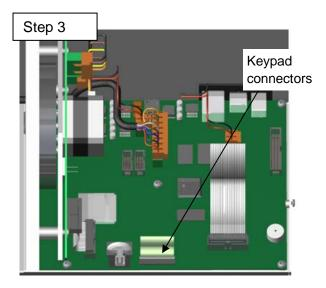
Remove the keypad connector to the connectors on the Main Boards as shown.
