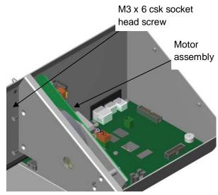
Replace the motor assembly by placing in position and inserting the 4x M3 x 6 csk socket head screws
