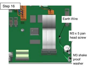
Attach the Earth Wire to the Main Board by replacing the M3 x 5 pan head screw and the M3 shake proof washer as shown.
