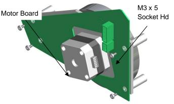
Attach the new Motor Board to the Motor bulkhead using 4x M3 x 6 cap socket head screws.
