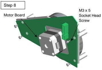
Remove the old Motor Board from the Motor bulkhead using 4x M3 x 6 cap socket head screws.
