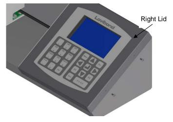
Replace the right lid carefully by replacing the 2x M3 x 5 pan head screws.
