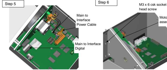
Remove the Main to Interface Power Cable and the Main to Interface Digital Cable from the connectors on the Main Board as shown.
