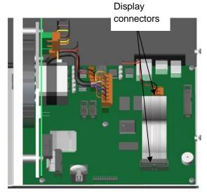
Replace the Display Connectors to the connectors on the Main boards as shown.
