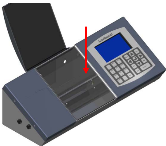
Replace the sample chamber taking care that the cables remain under the sample chamber then close the lid.
