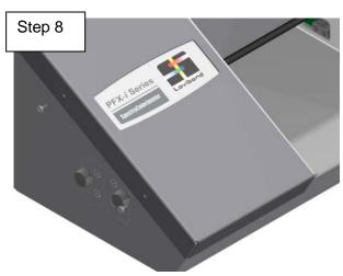
Replace the left hand lid, and tighten the 2x M3 x 8 socket head screws.
